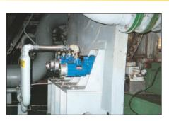
A multiple-starter application on a Clark *TCV-12 lowered air consumption by 40%* over competitive turbine starters originally applied.
